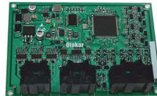
EV High Voltage Control Unit
